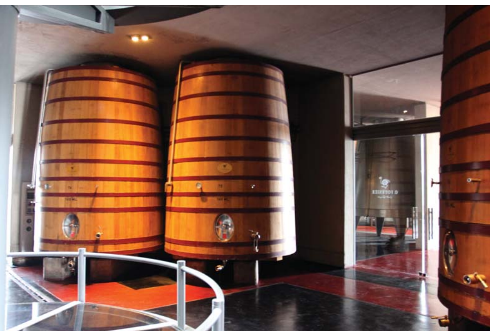
◀▲ The multilevel Cuv- erie - is equipped with fer- mentation tanks of both concrete, oak, and steel. These also vary in size from the small steel fermenta- tion tanks in their lab to the large concrete tanks in the cellar.
